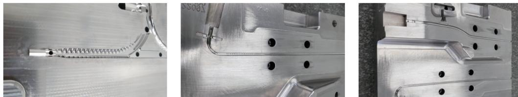
CORE STAVAX    PATTERN Minimum R R : 0.1    ROUGHNESS 20nm 이하
